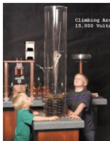
Figure 9 Climbing arc (or Jacob’s ladder)
